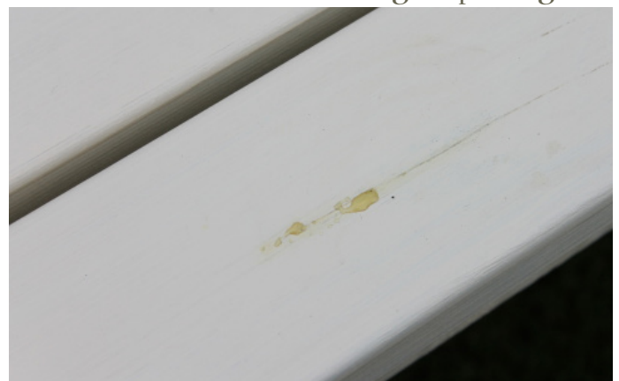
Only one small section on the table has experienced some resin bleed
